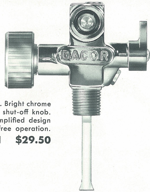
DEPTH COMPENSATING RESERVE VALVE Provides more reserve air at greater depths. Set for 300 P.S.I. reserve. Satin Chrome. RV-1 $29.50
